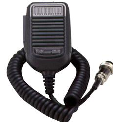
Hand microphone equipped with [UP]/[DOWN] switches. Same as supplied.
