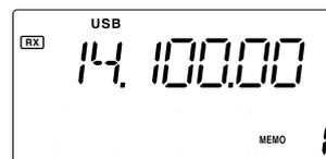
Changed frequency (14.123 MHz) does not appear and memorized frequency (14.100 MHz) appears instead.
