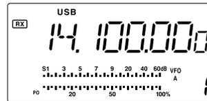
Rotating the tuning dial changes the frequency in 1 Hz steps.
