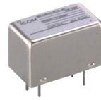
Contains a temperature-compensating oven heater and crystal unit for improved frequency stability.
