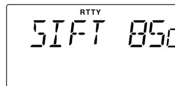
RTTY sift frequency is set to 850 Hz. 850, 425, 200 and 170 Hz are available.
