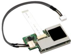
Provides AF DSP functions such as noise reduction and auto notch.
